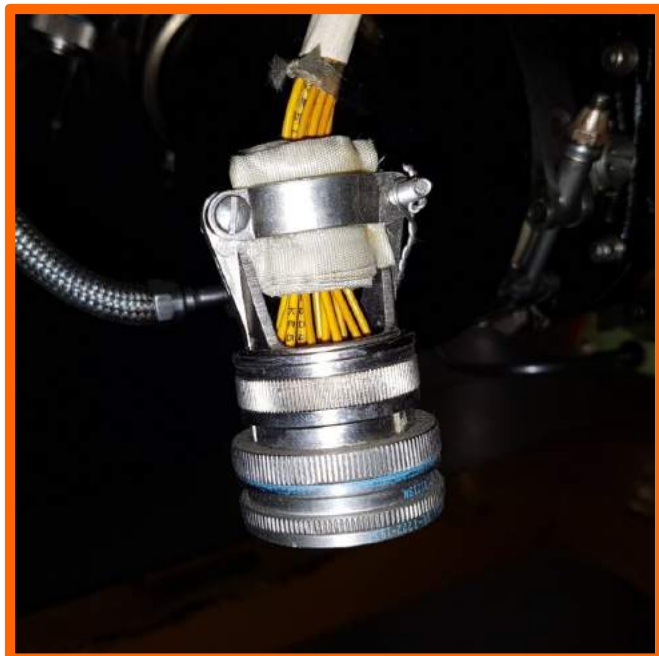
This tape is commonly used as a backshell clamp bushing
